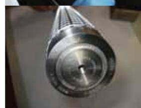
**DP Testing** - is a test for filters based on measuring the ratio of differential pressure across the filter to the flow of fluid passing through the filter. This measurement is a common factor in the specification of filters and the results obtained in this test can give an indication of the level of free flow in the filter.
