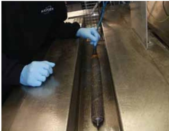
**The Flow Test** - is the open bubble point and is an extension of the bubble point test. The open bubble point is a relative measure of the mean pore size of a filter provided there are no other restrictions to flow or physical limitations. Since this point can vary from filter to filter and from filter media to filter media, PPSL introduced the 10LPM test several years ago which standardises the open bubble point test at an air flow of 10 litres per minute.
