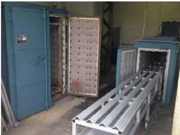
PPSL utilises two bespoke rate controlled ovens to effect the removal of a wide range of contaminants; from everyday paints and coatings, to modern chemical resistant polymers. The first oven in PPSL is a box oven able to accommodate parts up to 1.2 cubic metres. The second oven in PPSL is a screw cleaning oven able to accommodate parts up to 4m in length.
